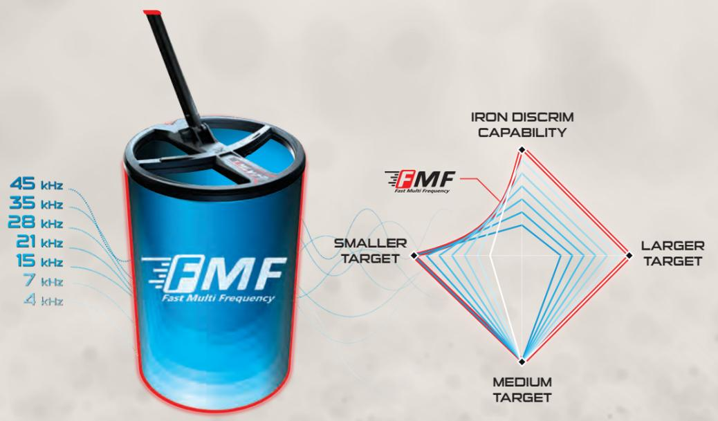
The above graphic illustrates the sensitivity and the iron discrimination capability depending on frequency and the advantage of Fast Multi Frequency programs covering a large spectrum of targets. This is only a basic schematic which can vary depending on the programs and real terrain conditions.
