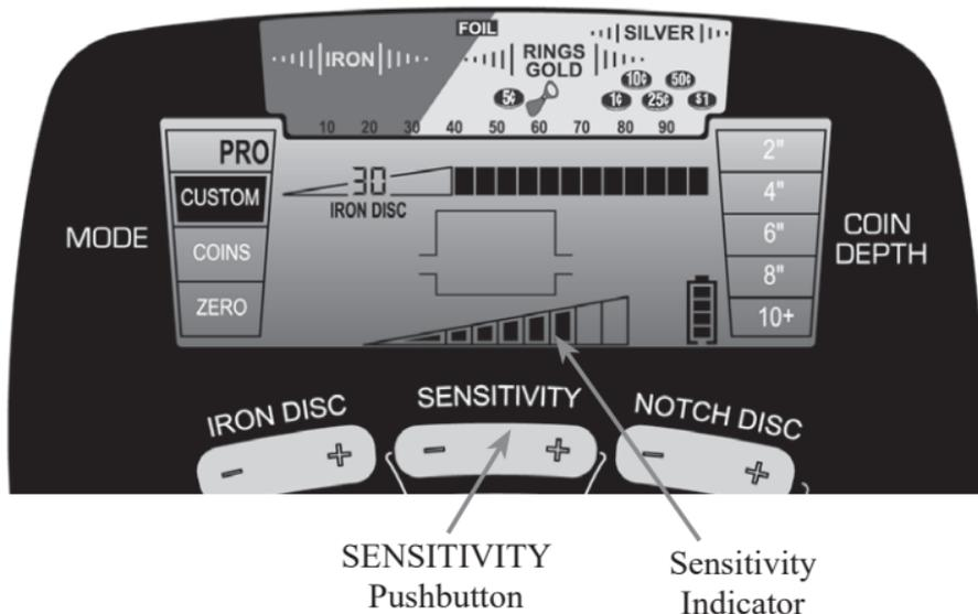
The *AT Pro* has eight (8) settings for sensitivity. Use the (+) or (-) SENSITIVITY buttons to step through the eight levels, which are continuously shown on the LCD.
