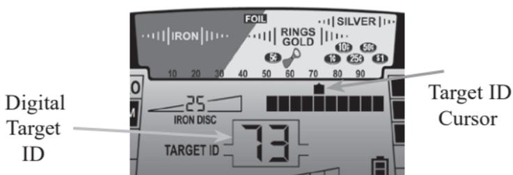
The AT Pro's Digital Target ID system provides a specific target value to help identify targets more precisely. Targets are identified on the LCD by number, with items near 1 being the most ferrous. The most conductive targets (such as thick silver) register closer to 99.
