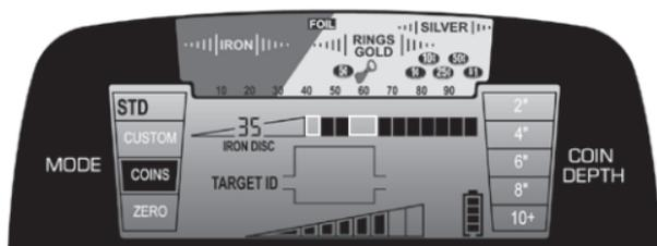
Designed to find most types of coins, jewelry, etc., while eliminating trash items such as iron and foil. High-Res Iron Discrimination level has been preset to 35 to exclude most iron targets. In addition, one pixel of foil and two pixels in the pulltab range have been excluded. Be aware that most pulltabs and pieces of tabs have not been eliminated from detection as these trash items have conductivities similar to small coins and jewelry.
