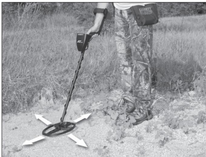
**Note:** For best pinpointing results, maintain a constant height above the ground (e.g. 1 inch) and ensure that the detector is properly ground balanced.
