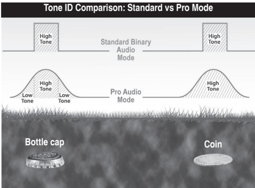
While in STD Mode, bottle caps, steel washers and other flat iron objects often sound like good targets, producing a high tone response. This is because the bottle cap's shape and flat surface resembles a coin which can trick the detector. In PRO Mode, however, the bottle cap will produce a very distinctive response with multiple tones. As shown, the bottle cap will produce a distinctive response of Low-High-Low as compared to the coin's response of only High tone.
