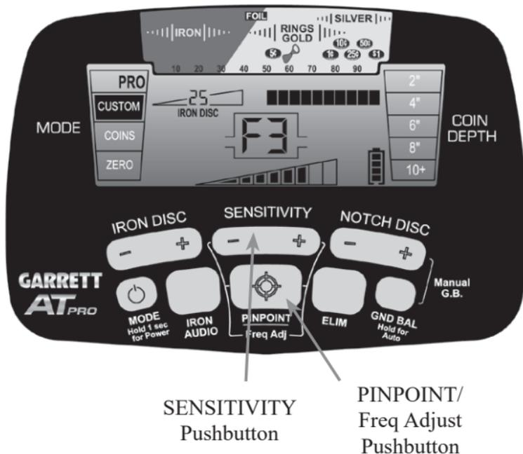
Use the PINPOINT/Freq Adj pushbutton in conjunction with the (+) or (-) SENSITIVITY pushbuttons to adjust frequency.
