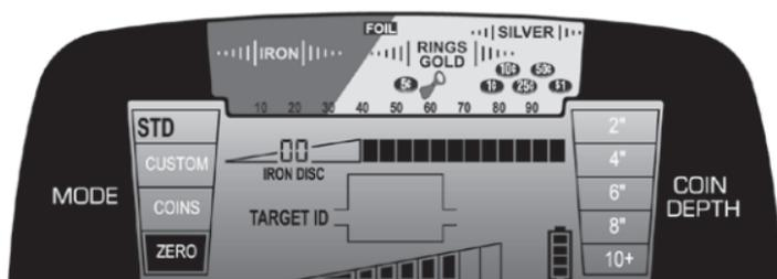
Designed to detect every type of metal; use ZERO mode to find all metal items or when the material of the desired object is unknown. All 12 discrimination pixels are switched on and High-Res Iron Discrimination is set to 0 (zero)—indicating that no metal targets have been eliminated.
