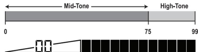
IRON AUDIO ON: With zero discrimination utilized and with Iron Audio ON, *AT Pro's* low tone is eliminated. The mid-tone extends down to 0.
