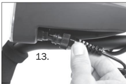
13. If desired, attach headphones to the 2-pin connector of the Control Housing. After lining up the connector pins, press the connector in firmly, yet carefully, until the O-ring is felt to be fully inserted.
