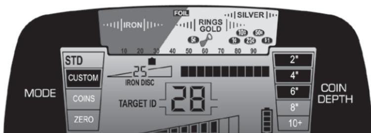
In Illustration 2, the same iron nail is laying above a good coin target. Since the Iron discrimination level is set to 25, the nail by itself would not be detected; however, the two objects have a combined conductivity of more than 25.
