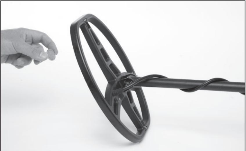
For bench testing, place the searchcoil on a flat, stable, non-metallic surface that is several feet from other metallic objects.
