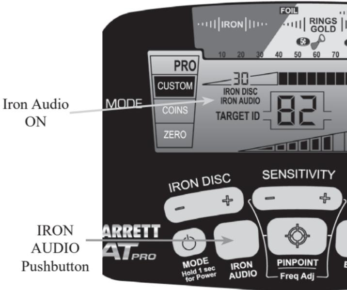
Press and release the IRON AUDIO pushbutton to switch the Iron Audio feature ON/OFF. When this feature is on, the words "IRON AUDIO" appear on the LCD (as shown in the illustration above). The Iron Audio feature can be used in any of the AT Pro's six modes.
