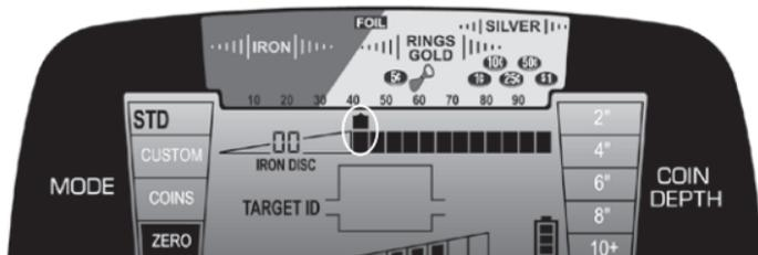
Use the NOTCH DISC buttons to position the Target ID Cursor above the pixel you wish to eliminate (see above illustration). Use the ELIM pushbutton to delete this pixel from the Lower Scale (see below). This item is now rejected.
