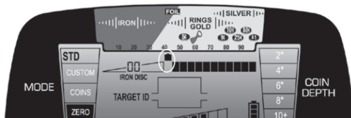
The second method of modifying the Notch Discrimination pattern involves the use of only the ELIM pushbutton. When an unwanted target is audibly detected while hunting, simply push the ELIM button to create a notch at that Target ID Cursor. The next time the *AT Pro* encounters the same trash item, it will not produce an audible signal.
