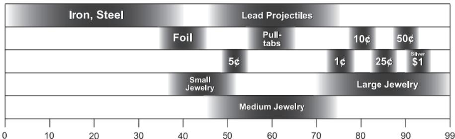
Note: Target values can vary based on the orientation of the target in the ground, amount of ground mineralization, etc. It is important to practice in the field to learn how these factors can affect Target ID.
