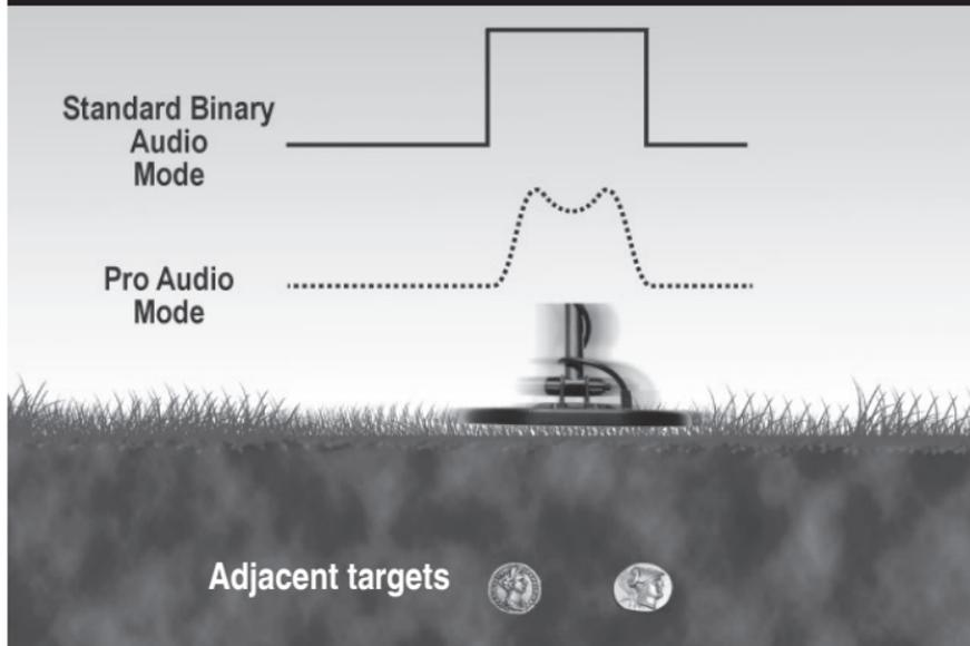
These two adjacent coins would produce one strong signal while in STD Mode. In PRO Mode, the proportional audio provides two peaks of audio response to allow the user to identify multiple targets.
