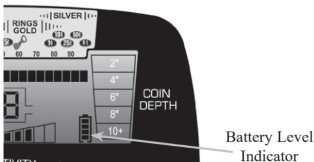
**Battery Replacement**—The *AT Pro* is operating with fresh or fully charged batteries when 4 illuminated bars on the **Battery Level Indicator** (see above) are displayed. The detector will maintain full performance until the batteries need to be replaced. Replace batteries when there is only
