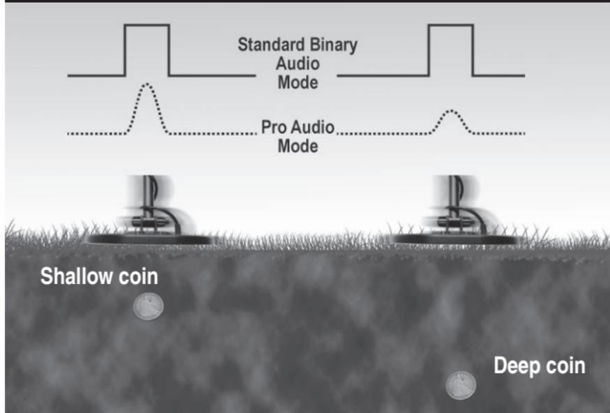
Notice the differences in Standard binary audio versus PRO audio in the two target scenarios above. The binary audio gives a solid, consistent beep for both the shallow and the deep coin. In contrast, PRO Mode's proportional audio provides a stronger signal for the shallow coin and a softer signal for the deeper coin. The actual profile, or signature, of the target's response is heard, thereby providing more information.
