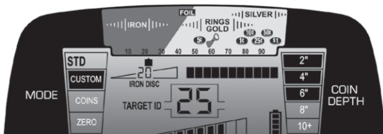
In the illustration above, the AT Pro is operating with an IRON DISC setting of 20. The nail seen in Illustration 1 (on page 25) registers from 10 to 25 on the Digital Target ID scale. To eliminate the nail from detection, increase the iron discrimination level to 25 using the IRON DISC (+) pushbutton.
