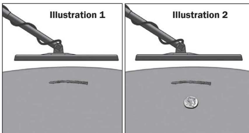
Iron targets, such as the nail shown in *Illustration 1*, can sometimes mask a good target's signal. If too much iron discrimination is applied, the good target (seen in *Illustration 2*) can be missed. Read page 26 to learn how to apply the proper amount of iron discrimination to eliminate the nail shown in *Illustration 1* and still detect the good target shown in *Illustration 2*.
