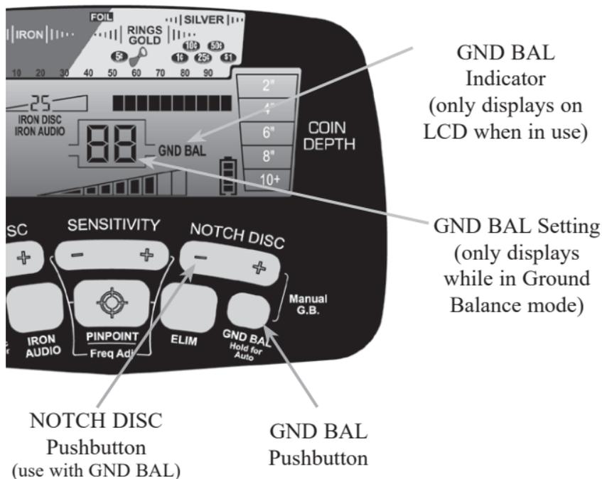
**GND BAL Pushbutton**—Hold for Automatic Ground Balance or use in conjunction with the NOTCH DISC pushbuttons for Manual Ground Balance.
