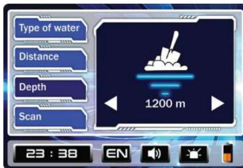
Use the left/right keys on the keyboard to change the desired depth. We also always recommend choosing the appropriate distance for the area in which we are searching, meaning it is not necessary to always choose the largest distance value available in the device.
