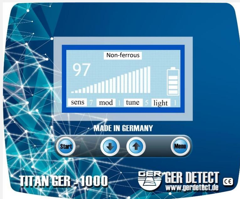
Adjust the sensitivity by the navigation buttons UP & DOWN.
