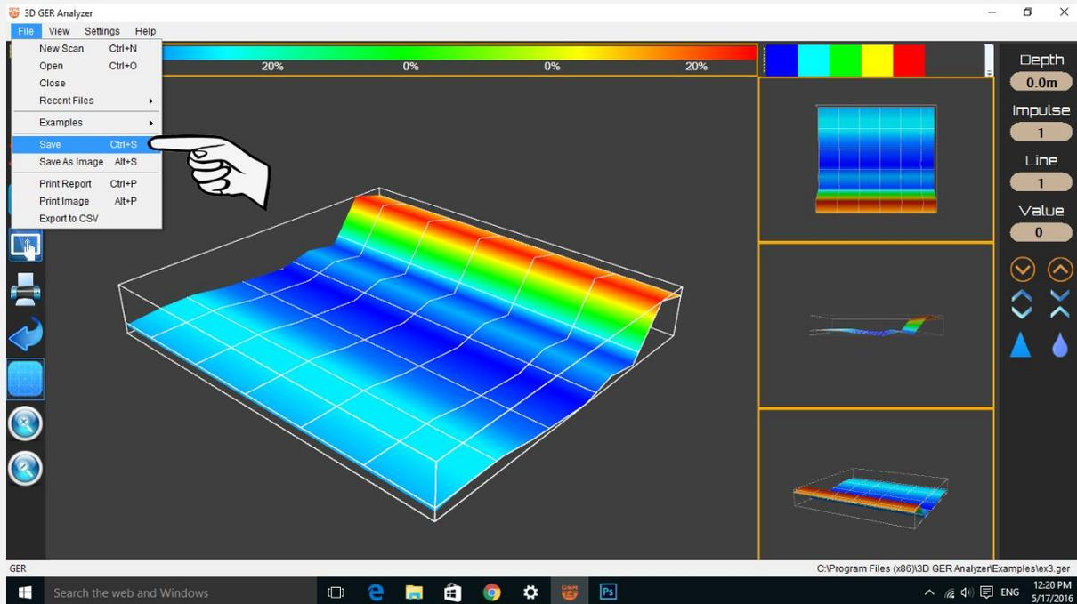
After you finish the scanning you can save the scan on the tablet as a project to be able to analyze again also you can save it as a photo
