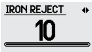
A high level of Iron Reject is very aggressive, but very effective at blanking ferrous targets. With a high setting some small desirable targets (e.g. gold coated in ironstone) could be mistaken as a ferrous target. This setting should only be used in very high trash areas, or when using the detector in lower mineralisation when searching for coins and relics.
