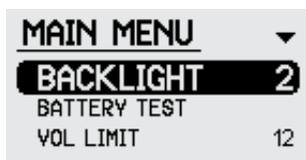
In low lighting conditions the LCD can be backlit. You can select how long the backlight stays on for once activated. Between settings one and six the time-out period is in increments of 10 seconds.
