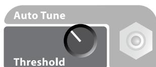
Threshold is the constant audible background tone or 'hum' produced by the detector. The Threshold is your reference point and lets you know what the coil is sensing, whether it may be a target, ground noise, or electrical interference, so it is important to set the threshold so it can be heard.
