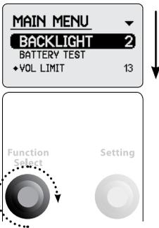
Turn the **Function Select** control right to scroll down the list. The currently selected function is highlighted.
