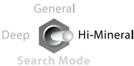
The GPX 4800 has three Search Mode switch positions: Deep, General and Hi-Mineral. The GPX 5000 has three Search Mode switch positions: Deep, General and Custom. Custom Mode is an open position which allows for the selection of one of the four additional Search Modes (p. 60), via the rear panel and LCD menu.
