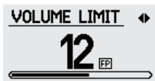
Volume Limit sets the maximum level of sound emitted by the detector when a target is detected.
