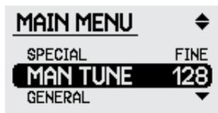
So that the detector experiences the least interference for the current environment, the search channel can be changed automatically by the Auto Tune button on the control panel, or manually in the Manual Tune (p. 59) setting via the LCD menu.
