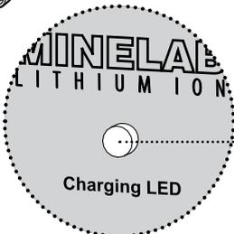
The colour scheme of the tri-colour LED (p. 20) will indicate the status of the charging process.
