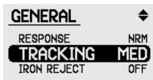
Tracking Ground Balance is the preferred setting when searching in highly variable mineralisation. Tracking Ground Balance automatically measures the ground mineralisation and adjusts the Ground Balance as necessary, to maintain stability and detection depth. The speed of the Tracking can be changed to suit the degree of variable mineralisation.
