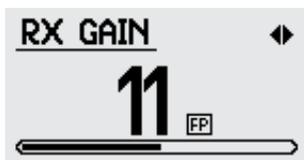
The Rx Gain function allows the GPX Series to be optimised for differing conditions; controlling the sensitivity of the detector to its environment and targets.
