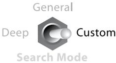
The Search Mode switch, on the Front Control Panel, provides access to a number of detecting modes that you can use in different circumstances. Deep and General are two of the positions on the Search Mode switch, and the third position is Custom. Custom allows you to select one of the four Custom Search Modes from the LCD menu.
