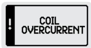
Avoid turning the detector On and Off repeatedly. If this happens the Coil Overcurrent screen will appear. Turn the detector Off and wait for a short time before turning the detector On again.
