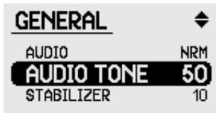
Audio Tone is the pitch of the Threshold emitted by the detector.
