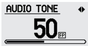
A high Audio Tone setting may help identify small targets from ground signals, but a low Audio Tone setting may allow deep target signals to stand out.
