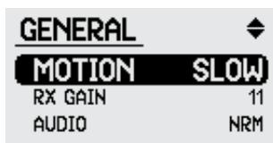
The speed at which you sweep the coil has an effect on target response time and Ground Balance adjustment. Matching your preferred coil sweep speed with the corresponding Motion setting can reduce noise and improve target signal responses.
