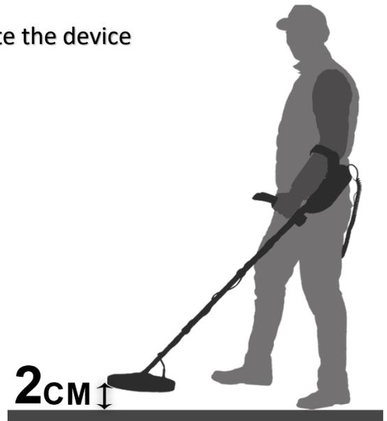
The distance between the search coil and the ground should be around **2 CM** while be doing the search to reach as much depth as possible.
