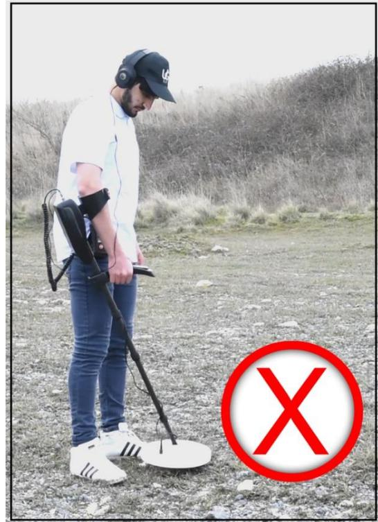
Avoid the continuous friction of the coil with the ground and rocks.
