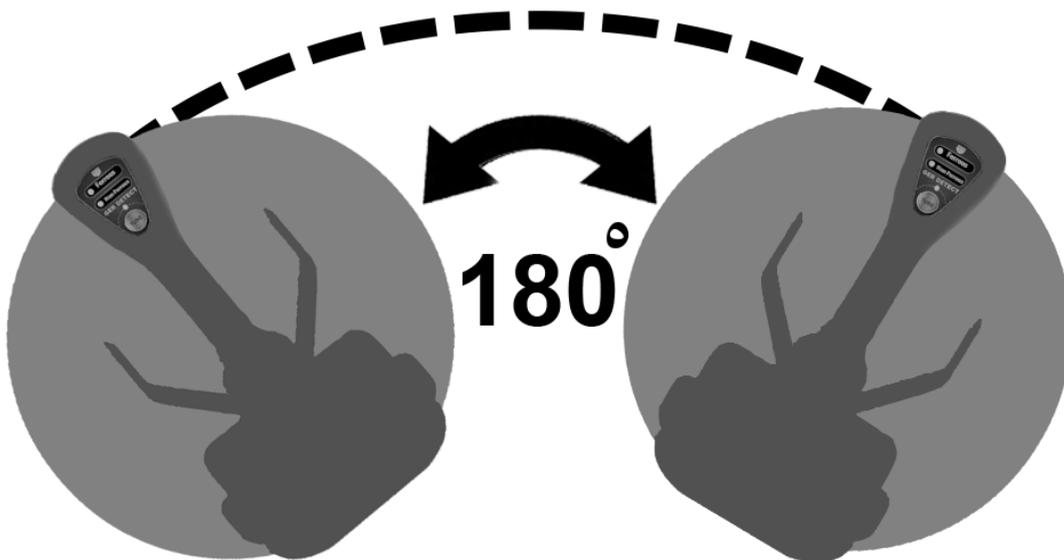
Start the search by moving the device right and left at a normal speed
