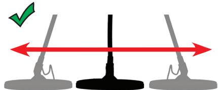
The search coil must be parallel to the ground at all times.
