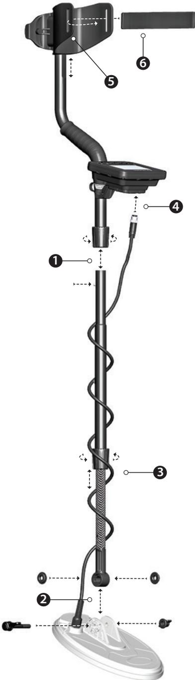
(1) To attach the middle rod with the upper S-rod, loosen the twistlock. Press down the pin and engage the pieces together and tighten the twist lock after the pin is clicked into the hole.
