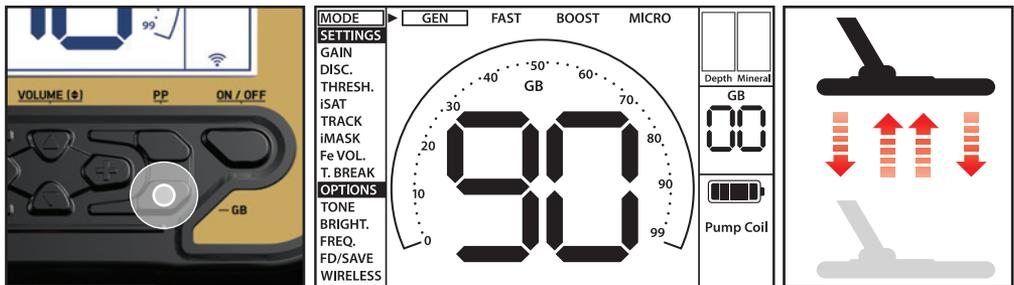
3) Continue until a beep, indicating the completion of ground balance, is heard. Based on ground conditions, it usually takes about 2-4 pumps for the ground balance to be completed.
