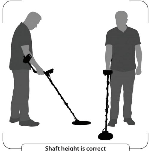
Adjust the height of the shaft so that you are standing in an upright position, your arm is relaxed and the search coil is approximately 5cm (~2") above the ground.
