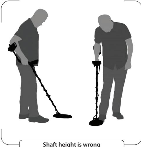
It is very important to adjust the shaft to your height correctly to be able to search without discomfort and fatigue.
