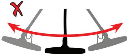
It is important to keep the search coil parallel to the ground in order to get accurate results.
