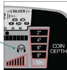
Once paired, if the headphone/receiver is switched off or moved out of range, the *AT Max* will search and attempt to reconnect to the receiver for 30 seconds, indicated by a flashing icon. If the connection is not reestablished during this time, the *AT Max* will switch off its wireless transmitter. It will be necessary to switch the *AT Max* off and then on again to initiate a new 30-second search.
