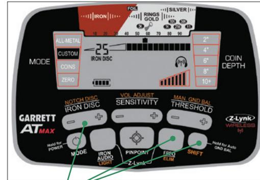
Press SHIFT, then use the NOTCH DISC buttons to position the Target ID Cursor above the pixel you wish to eliminate (see illustration). Use the ELIM button to delete this pixel from the Lower Scale (see below). This item is now rejected.
