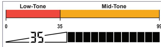
**IRON AUDIO ON:** In All Metal Mode with this example, iron targets below 35 are now heard with flanking low tones and targets above 35 produce a clean medium tone.
