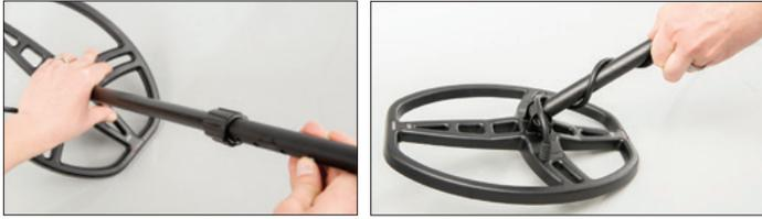
Insert coil connector into the 4-pin connector of the control box by lining up connector pins. Press firmly, yet carefully, until the O-ring is felt to be inserted, and hand-tighten.
