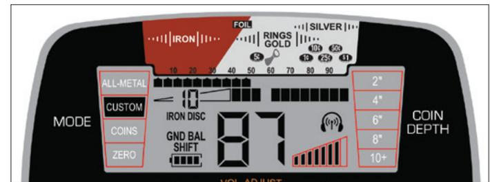
Ground Balance values above 75 increase in quarter-points of resolution. The above illustration indicates a Ground Balance value of 87.5. Above the solid numeral 87, each quarter-point of value is indicated by five blocks of pixels on the upper scale.
