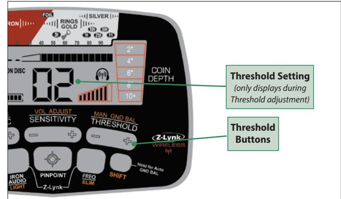
Threshold is the constant background “hum” that is added to the target response. Press a Threshold button once to display the current setting. Press the (+) or (-) Threshold buttons again to select from 33 levels, ranging from -9 up to +23.
