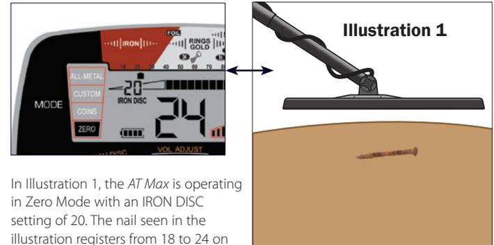
In Illustration 1, the *AT Max* is operating in Zero Mode with an IRON DISC setting of 20. The nail seen in the illustration registers from 18 to 24 on the Digital Target ID scale. To eliminate the nail from detection, increase the iron discrimination level to 24 using the IRON DISC (+) button.
