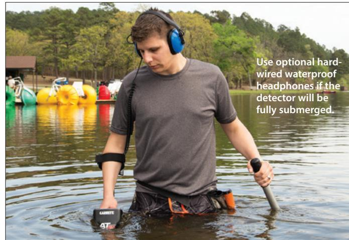
Use optional hard-wired waterproof headphones if the detector will be fully submerged.
