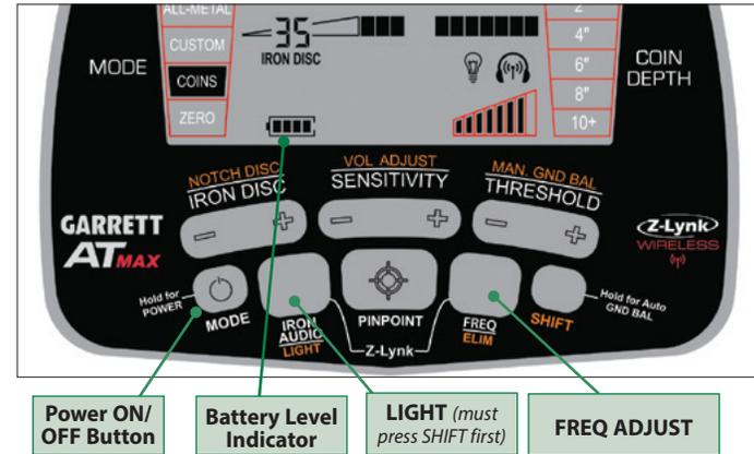
**Power ON/OFF**—Hold this button for 1 second to switch power ON or OFF.
