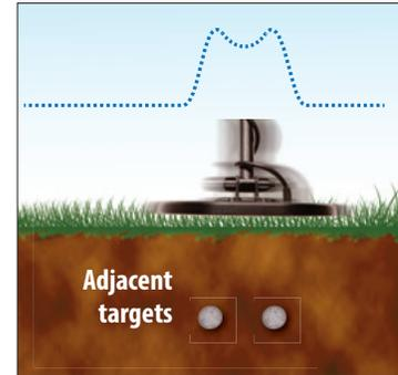
Example A: Adjacent targets can often produce a single strong signal with many metal detectors. The fast recovery of the *AT Max*, however, will provide two peaks of audio response to these adjacent coins. These multiple audio responses provide the experienced user with more target information.
