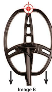
Once the target signal drops off (both audibly and on the LCD meter), shallow targets should be located immediately in front of the searchcoil's tip (see *Image B*). Deep targets will be under or just inside your searchcoil's tip. This is because the conical shape of the searchcoil's detection field begins bending in slightly as the depth increases.
