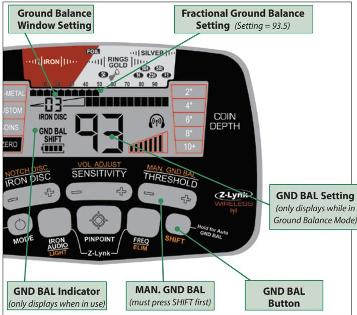
**GND BAL Button**—Hold the SHIFT button for Automatic Ground Balance or, for Manual Ground Balance, press and release SHIFT and then use the (+) and (-) MAN. GND BAL buttons.
