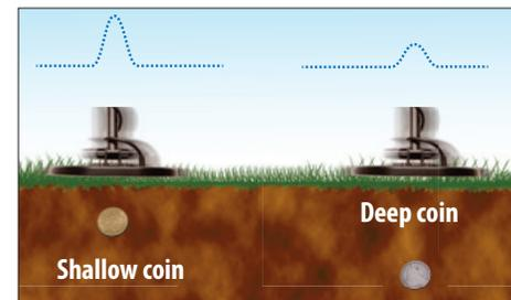
Example B: Notice the different target response provided by the *AT Max*'s proportional audio in regards to target depth. The shallow coin target offers a stronger signal, while the same-sized deep coin provides a softer signal.
