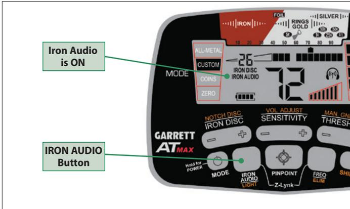
Press and release the IRON AUDIO button to switch the Iron Audio feature ON/OFF. When this feature is on the words "IRON AUDIO" appear on the LCD (as shown in the illustration above). The Iron Audio feature can be used in any of the AT Max's four modes. Its functionality in the three Discrimination Modes versus the All Metal Mode will be discussed separately.
