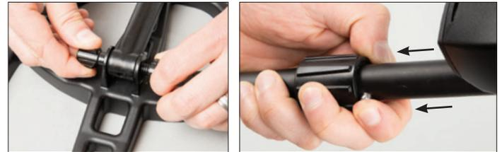
Note: The spring clip must be engaged in the FIRST stem opening in order to access battery compartment.
