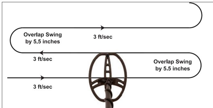
In order to fully search an area, overlap the swings of your searchcoil by half the length of the coil (about 5.5 inches). Sweep the searchcoil in a straight line or with a slight arc at a sweep speed of about 3 ft/sec.
