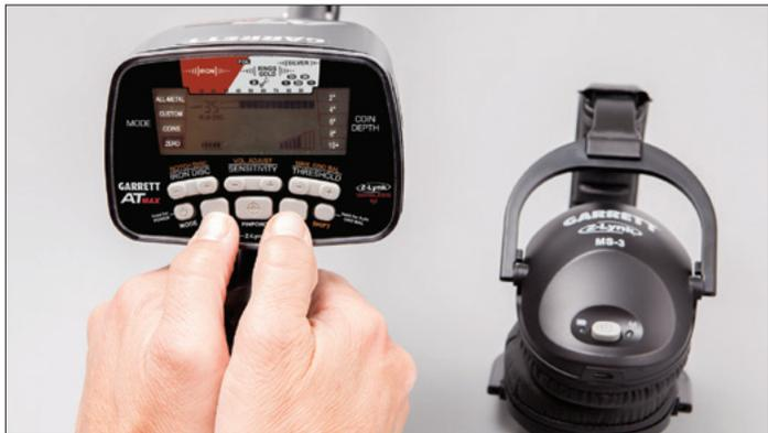
**PAIRING:** Switch on headphones and hold within 2 feet of *AT Max*, then press and release Z-Lynk buttons (IRON AUDIO and FREQ) simultaneously.
