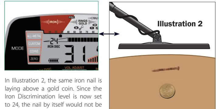
In Illustration 2, the same iron nail is laying above a gold coin. Since the Iron Discrimination level is now set to 24, the nail by itself would not be detected; however, the two objects (nail and gold coin) have a combined conductivity of more than 24.
