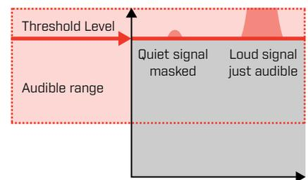
If the Threshold Level is too high, it can make faint targets more difficult to hear above the threshold hum.
