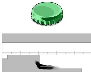
Bottle cap B is more difficult to reject as iron, and requires a higher Ferrous Limit Lower preset setting.
