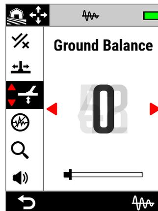
The Ground Balance value will update automatically as it tracks to changing ground conditions.
