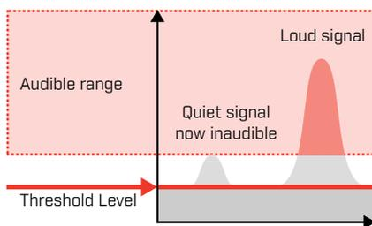
If the Threshold Level is too low, the variation caused by a small or deep target may be inaudible.
