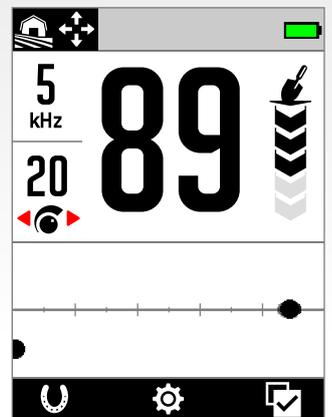
This example shows the detection of a coin and a nail in Multi-IQ+, then again using a single frequency. While the coin's Trace and ID remain very similar, the ferrous nail appears on the far lower left when in a single frequency.
