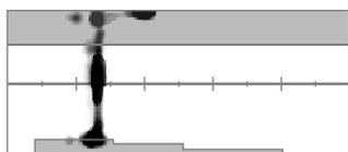
A hammered coin (low conductor) buried deep in highly mineralised soil, showing a solid Target ID, but uncertain ferrous characteristics due to being mixed with the ground signal response.
