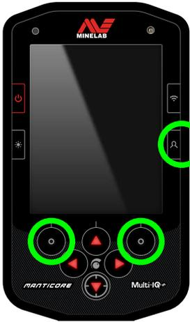
The **Side Soft Key** is the bottom right Side Button on the Control Pod. Actions assigned to it do not display an icon until the Soft Key is pressed.
