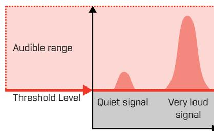
If the Threshold Level is just right, it should sound like a faint audible hum. This emphasises variations in signal response making targets easier to hear.
