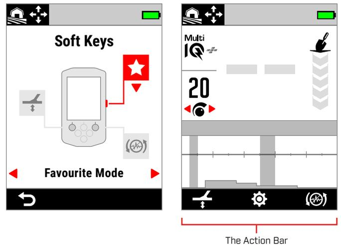
The Soft Keys Selector and the resulting Action Bar on the Detect Screen.
