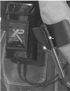
Insert the control box into the hipmount bag.
