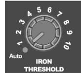
The GMAXX II is still a "multi-tone" detector, but users can now adjust the iron level setting by using the IRON THRESHOLD potentiometer.
