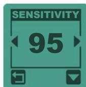
Determines the device's sensitivity level from 0 to 99.
