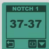
The Notch complements the discrimination: it enables a "target window" to be rejected whereas discrimination rejects all targets below a selected threshold. For example, if you detect an undesirable target in the ground, you can decide simply to reject the corresponding conductivity group and continue to detect targets with a conductivity higher or lower than those in the rejected group.
