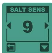
In addition to the general sensitivity setting, the «SALT SENS» setting has the advantage of reducing false signals, typically linked to seawater, unlike the general sensitivity which acts on all targets and all signals. When searching wet sand or surf, always use the SALT SENS setting as a priority rather than the general sensitivity. The general sensitivity should be reserved for cases where the instabilities come from electromagnetic interference (EMI).
