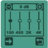
Over and above a simple low/high audio setting, the equalizer can correct the acoustics of headphones over four bands to match them to your hearing preferences. You can thus set the low tones to around 150 Hz, the medium low to around 450 Hz, the medium high to around 2000 Hz and the high to around 4000 Hz.
