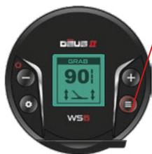
From the Grab menu, you can calibrate the ground effect at any time by holding the key down while you pump the coil on the soil until the ground audio signal is attenuated and the value is stabilized.
