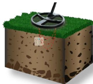
To narrow the field of detection and improve the target location: Position the coil close to the target but not on the center. Press
