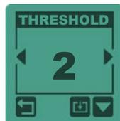
This feature is used to set the amplitude of the background sound threshold. Threshold will go silent when passing over rejected targets.
