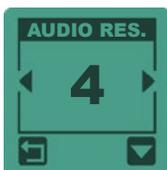
Audio Response enables you to amplify the volume of deep targets. It gives the impression of greater power, but does not provide any additional depth as this setting only affects the sound curve (the dynamic range of sounds). Lower Audio response levels give a good perception of depth.
