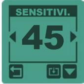
The MI-6 has 50 levels of sensitivity via the **WS6 MASTER**. Press **-** and **+** to increase or decrease the MI-6 sensitivity.
