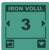
Adjust the volume of the low-pitched tone which has a lower value than the discrimination setting, which normally means iron.
