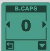
B.Caps rejects the rusty beer and fizzy drink bottle caps effectively. Make sure you activate it on the beach, in parks and polluted zones. B.Cap reject also assists with rejecting some types of iron which is usually difficult to discriminate, such as ferrous cartridges, ferrous rings and some larger mis-shaped ferrous.
