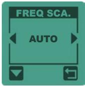
This function activates an automatic scan of the detecting frequencies and indicates a clear channel with the least interference at every change of program or every change of frequency in the MONO program. The frequency scan is particularly fast on **DEUS II**, however it will slow your navigation by 2 sec. when changing program.
