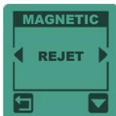
When searching magnetic ground such as black sand, deep targets may be masked because their values are similar to the soil values. The Magnetic Ground setting allows you to accept medium tones generated by the ground, ferrite, meteorites as well as distant targets that are usually masked.
