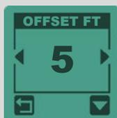
the OFFSET FT feature allows the user to shift the "Full Tone" audio frequencies of targets with a signature just above the Discrimination threshold, in order to better differentiate them audibly from iron.
