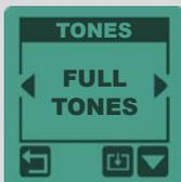
Full Tones assigns tones specific to each target index in proportion to its conductivity. The higher the conductivity index of a target, the higher the signal.
