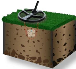
Move the coil slowly across the target. The loudest sound and highest audio pitch indicates the target position.
