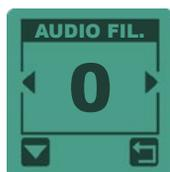
This function is to filter the audio and produce softer and more fluty sound, especially when target is at the detection limit. At depth the signal will be less scratchy. In some situations, Audio Filter can gain a little extra depth.
