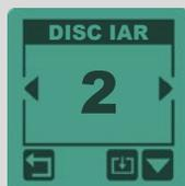
Programs 8 GOLD FIELD and 9 RELIC FIELD use another discrimination method, called IAR (Iron Amplitude Rejection). This allows rejection of ferrous items according to their distance from the coil.
