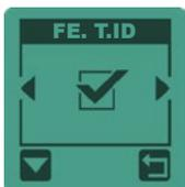
This function turns on/off the visual target IDs for targets that fall below the discrimination setting, for example when FE TID is set OFF you only see the TIDs above the discrimination adjustment even if you keep the Iron Volume ON.
