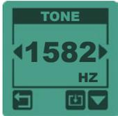
Modify the low/high audio tone of the **PULSE Mode** from 100 to 1582 Hz.
