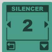
A few large iron objects or unusual shapes are often more difficult to discriminate. Iron objects often generate a few audible remnants of broken or inconsistent signals (crackling). Increasing the silencer applies a filter which eliminates the crackling caused by ferrous items.
