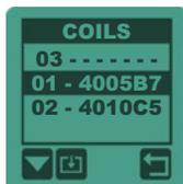
To switch off the coil LED and wireless headphones during use: In OPTION > COIL pairing, select your coil of choice as opposite and press the **+** key for 3 seconds. When switched off, this mode becomes deactivated and the LED return to normal operation.
