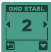
This setting can be adjusted from 1 to 3 and is used to define the level of ground instability / feedback you are prepared to tolerate.
