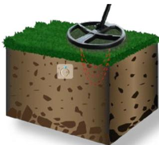
Position the coil barely off the ground and to the side of the target. Press
