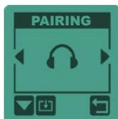
Press **OPTION >** **PAIRING**, with **-** or **+** Choose the headphone then press **↵** and switch on the headphones by holding the **-** key down for 8 s.
