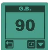
Press to access the G.B. (ground balance) and press 2 seconds to enter into G.B. settings.
