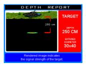
You can now begin by determining the dimensions of the target. To do this, move the coil towards the target. You will want to approach the target from the coil's side. Note that the front and rear parts of the coil are not used during measurement. Mark the first points at which you receive
