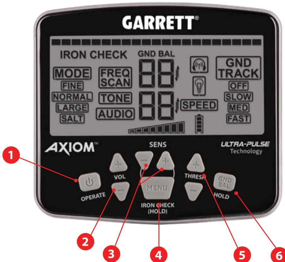
Note: Use the Plus (+) or Minus (-) above the Menu button to adjust any of the Menu options. Axiom automatically exits the Menu settings after 20 seconds with no activity; or, simply press the OPERATE button at any time to exit the Menu.
