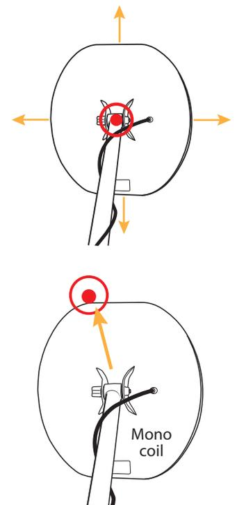
For very small, shallow targets, use either front corner of the mono coil to more precisely locate the target.
