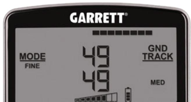
This detected target is causing the upper row of pixels to swing to the right, which corresponds with a target creating a high tone..
