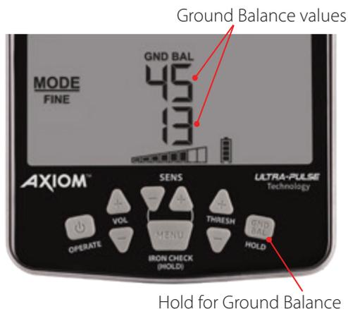
During a Ground Balance procedure, GND BAL will display on the LCD. Dual Ground Balance values are shown by the upper and lower 2-digit numbers.
