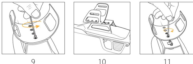
**Caution: Always power OFF your Axiom before changing searchcoils. Disconnecting and reconnecting coils while the detector is powered on could damage the searchcoil and/or the detector's electronics.**
