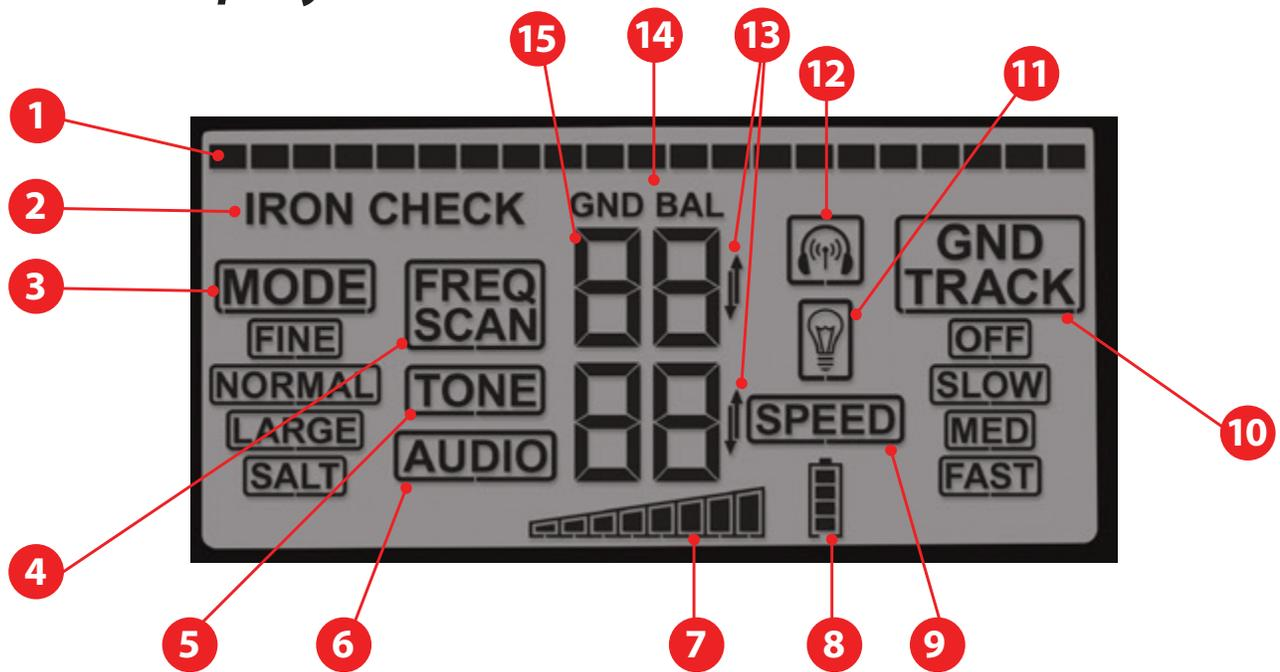
1. **Signal Strength Indicator**—directional bar graphs indicates both signal strength and polarity (i.e. high tones to the right; low tones to the left).
