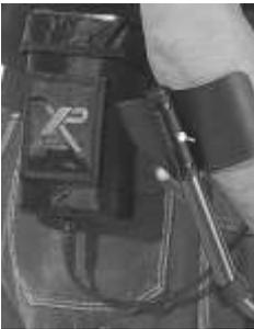
Insert the control box into the hipmount bag. Then insert the connector (female) in its panel connector (male) and screw it.
