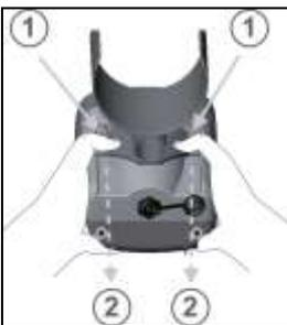
To remove the control box from the armrest, proceed as indicated below. Put your hands around the control box and press slightly with your thumbs on the side of the armrest (1).
